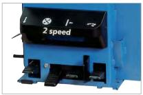
The pedal-controlled two-speed chuck (3-ph versions only) makes tyre service even quicker.
