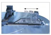
The sliding jaws allow to handle wheels from 10" to 26" (with optional jaws even up to 30").
